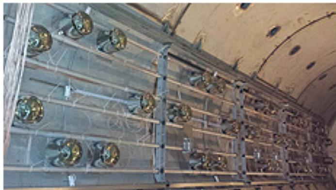
MicroBooNE's optical system, which captures and measures light resulting from particle interactions, was recently installed in the experiment's detector.
