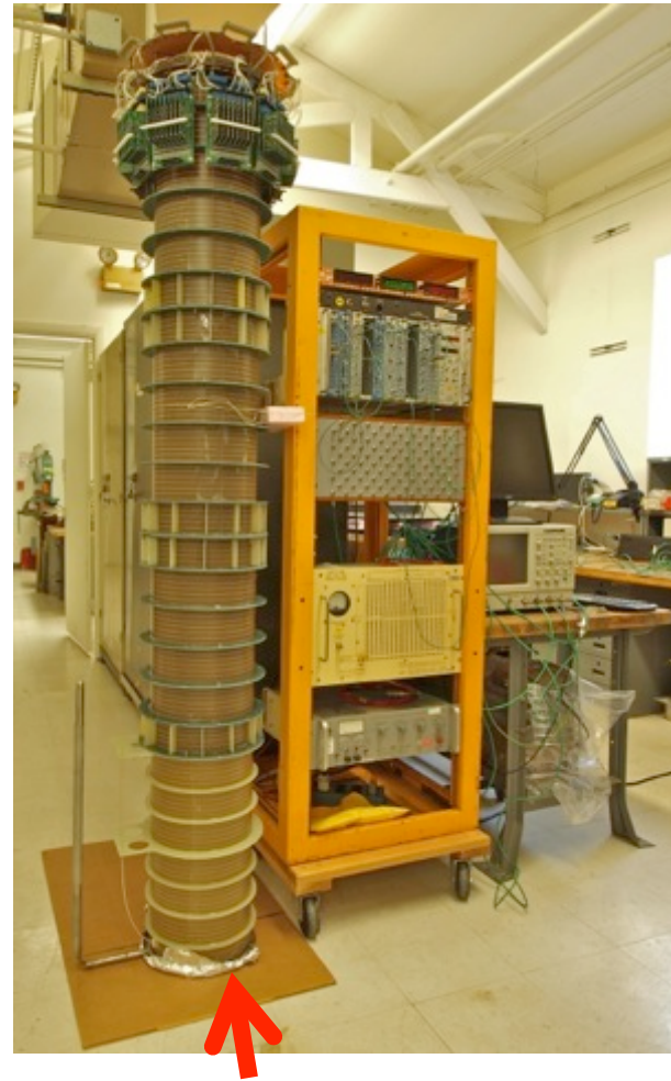
Long Bo TPC, equipped with electronics from MSU
