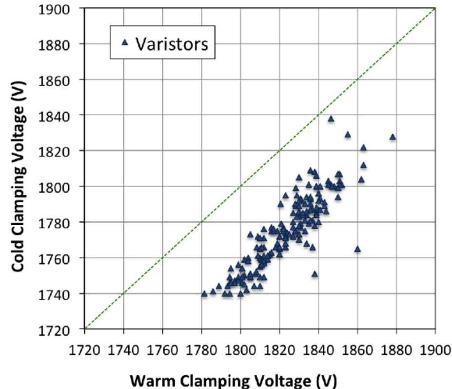
**Clamping voltage defined as  $V$  applied for 0.5 mA current draw**
