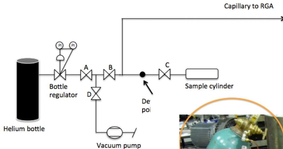
Built a setup at PAB to supply GDT contents in helium carrier gas to UGA
