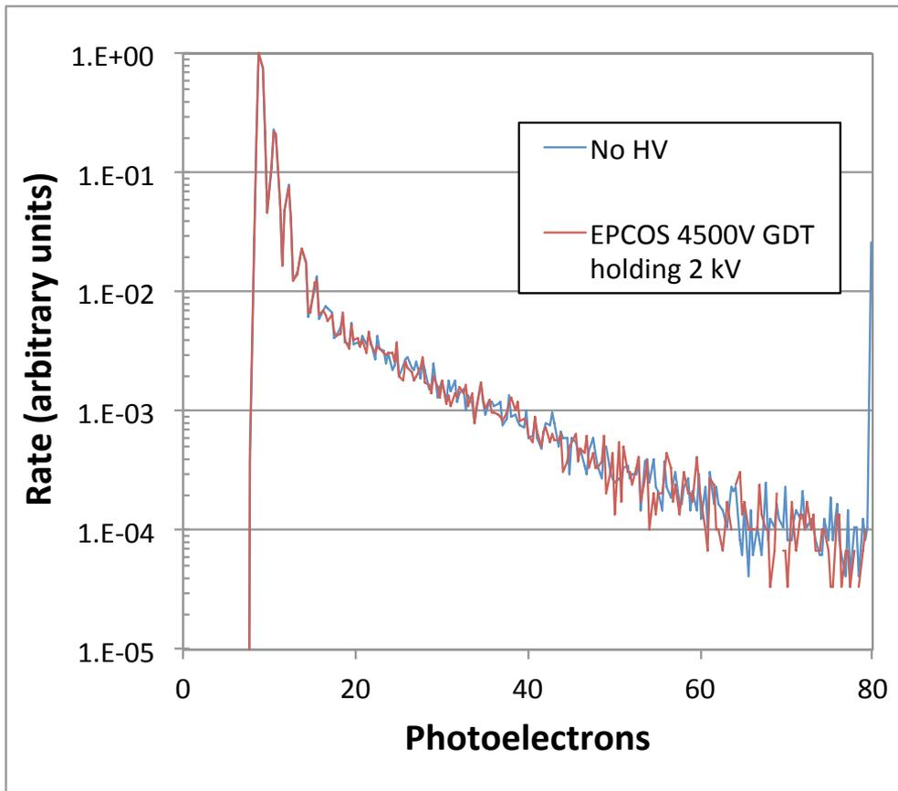
**No difference from HV-off cosmic spectrum, including in overflow bin.**
