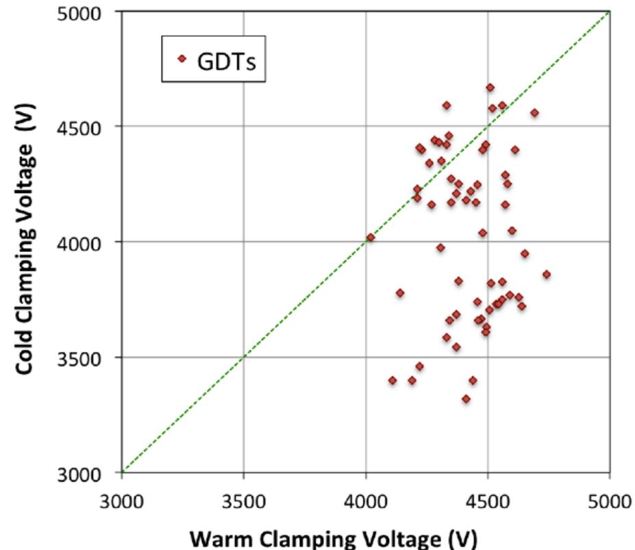
**Clamping voltage defined as  $V$  applied for device sparkover and power supply trip**
