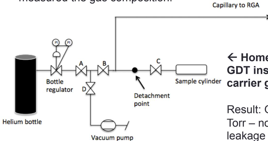
← Home-made setup for breaking open a GDT inside a pre-characterized helium carrier gas
