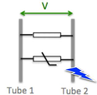
**With surge protection, the potential difference does not rise above the clamping voltage.**
