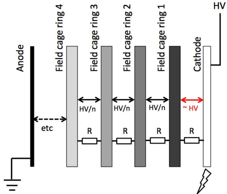
*The exact voltages evolved depend on **all** the capacitances in the TPC-Cathode-Cryostat system*
