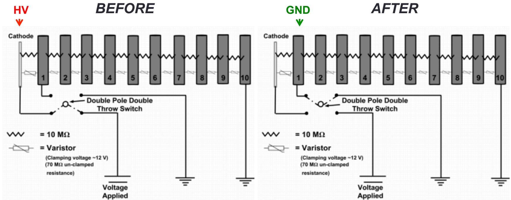
Figure 1: Schematic for our testing setup with the switch (a) charging the cathode and (b) simultaneously removing the voltage supplied to the cathode and grounding tube 1 (T1).
