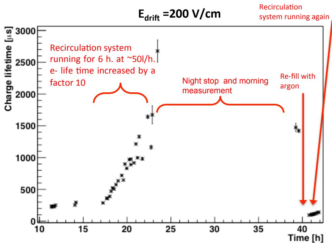
ARGONTUBE routine operation: 2.5 ms lifetime (0.12 ppb Oxygen equivalent)
