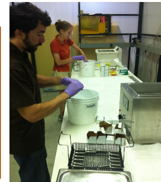
Small ultrasonic bath for cleaning hardware & small parts (Thanks Pete Simon)
